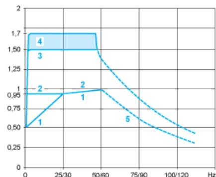
1 : Self-cooled motor: continuous useful torque (1)
